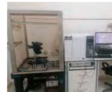
Figure 2: Schematic diagram and photo of a gas chromatograph coupled to an electroantennogram detector, used to identify the compounds in a sample that induces a physiological response from the insect antenna. The compounds that elicit a physiological response are good candidates for further investigation of behavioural activity.
