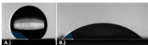
Figure 3: Contact angles for A) a water droplet without surfactant; B) a water droplet with surfactant.
